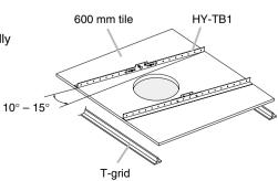
Step 2. Install the ceiling reinforcement ring supplied with the speaker.
