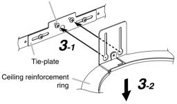
Reinforcement ring mounting screw
