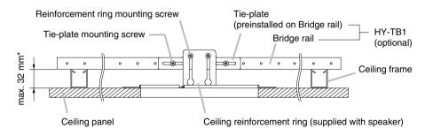
\* This length can be extended to up to 58 mm by turning the tie-plate upside down.
